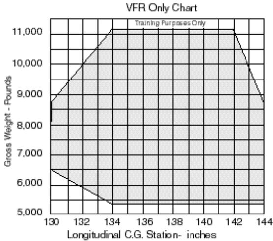
**Figure 15-2 Gross Weight Center-of-Gravity Chart**
