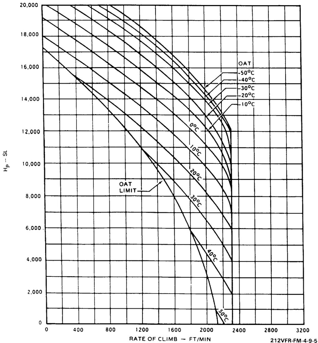
**Figure 15-14 Twin Engine Rate of Climb**
