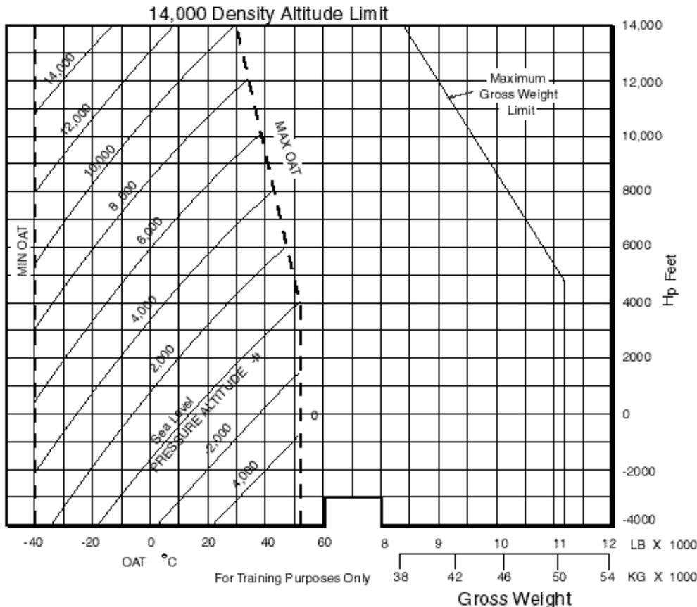
**Figure 15-1 Weight-Altitude-Temperature Limitations Chart**
