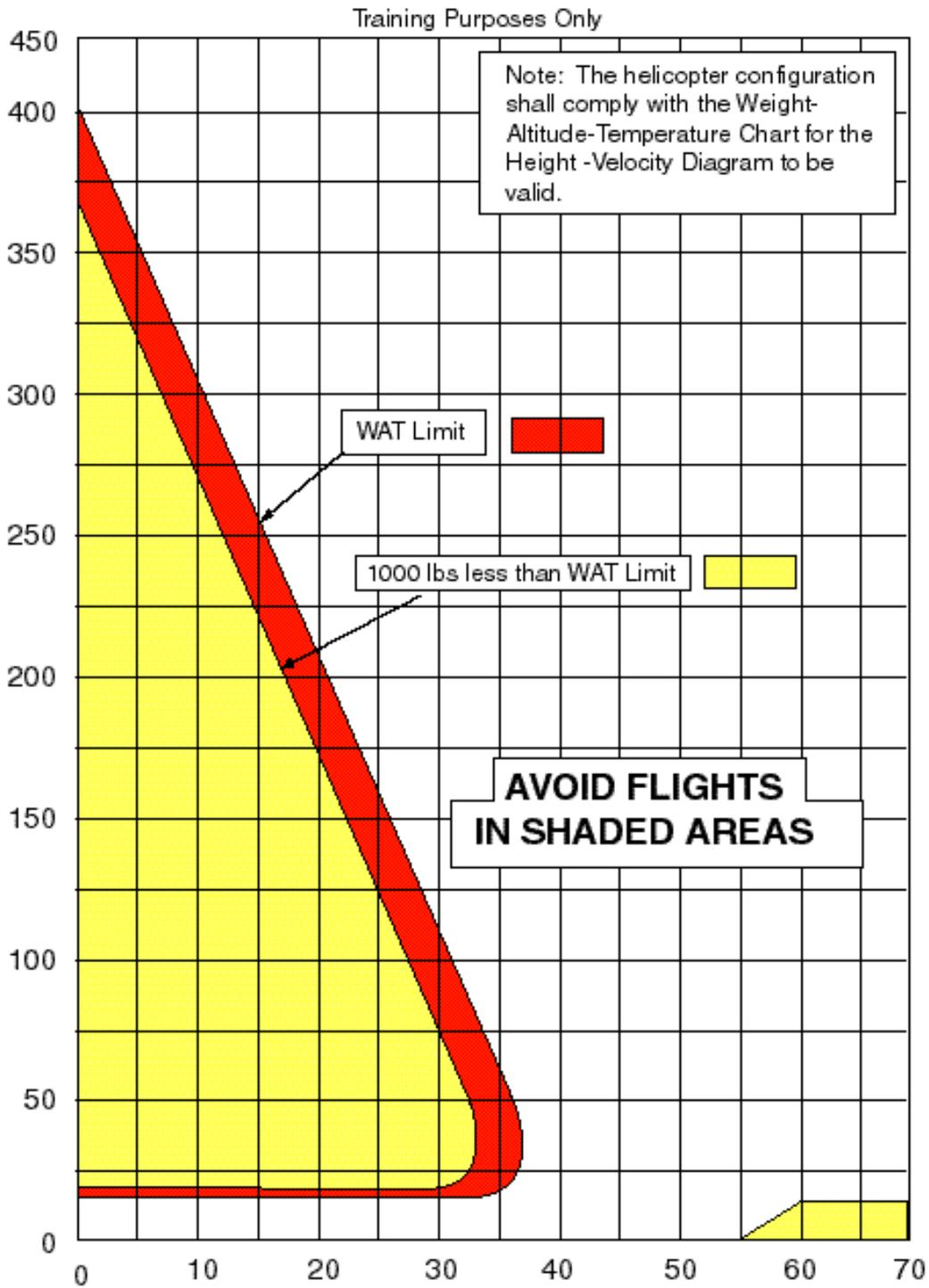
Figure 15-4 Single Engine Height Velocity Curve
