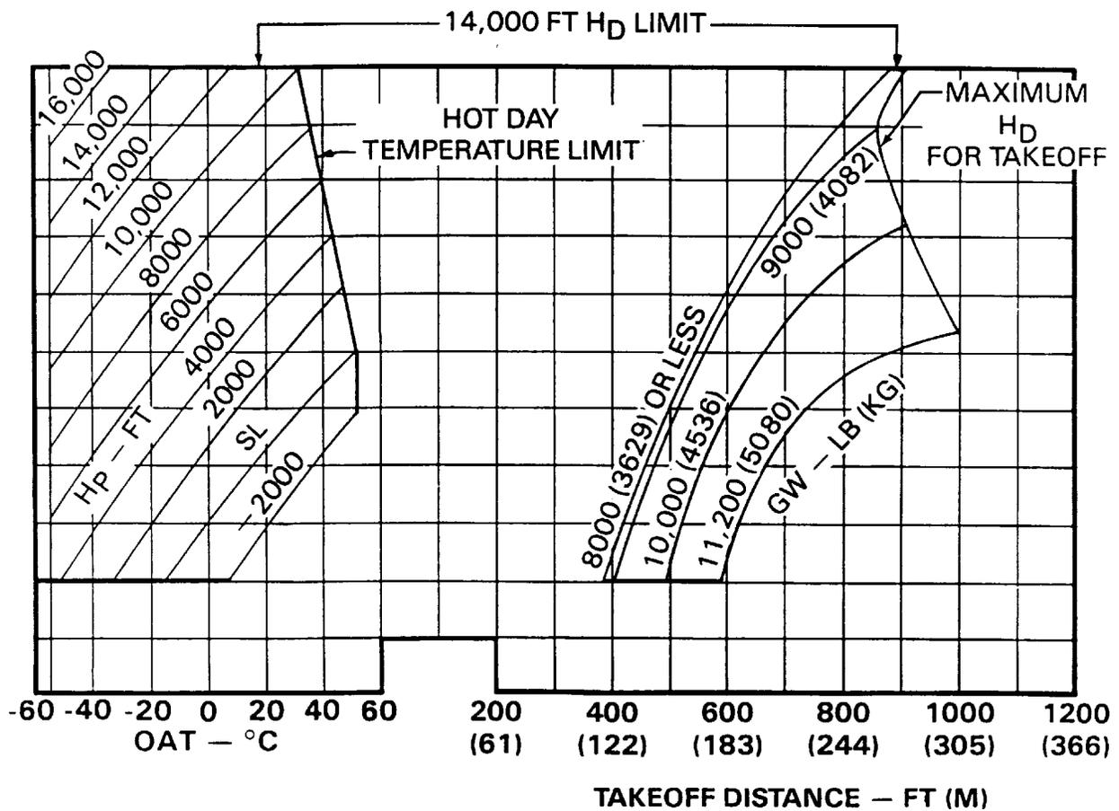
**Figure 15-12 Takeoff over a 50 Foot Obstacle**
