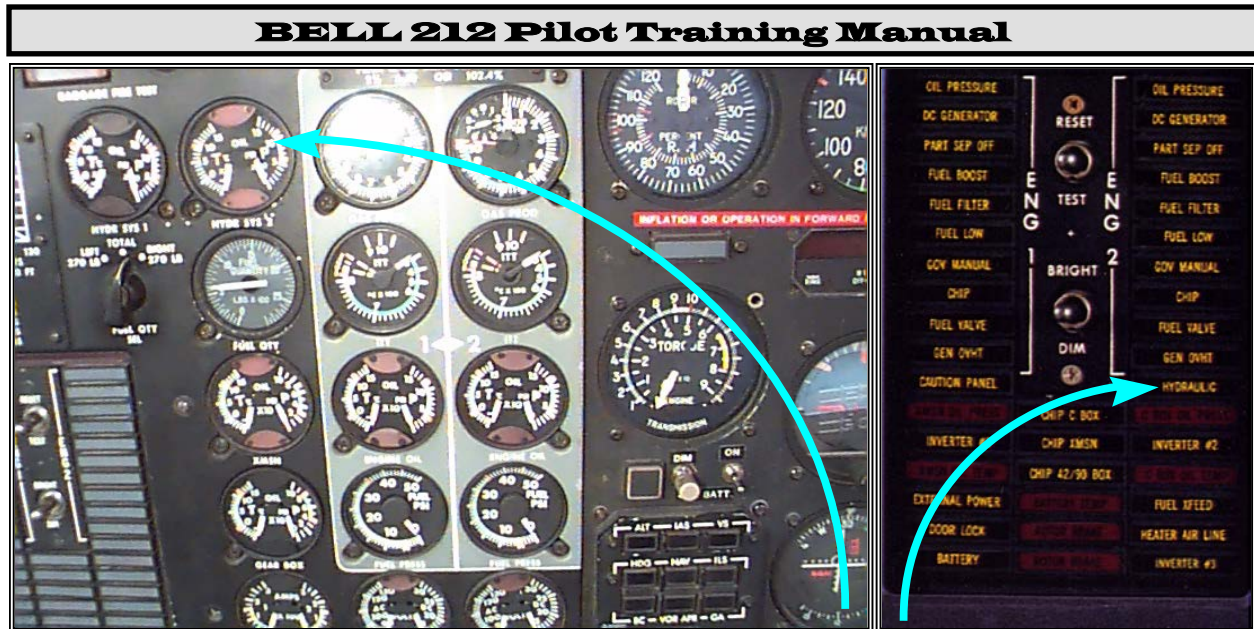
Figure12-8 Hydraulic System Cockpit Indicating Systems
