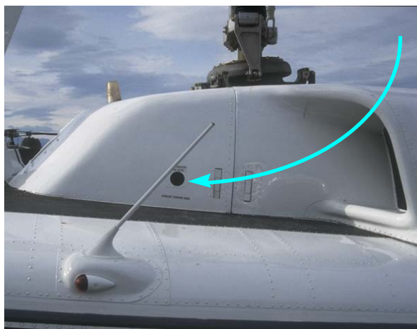
Figure 12-4b Hydraulic Reservoir View port in Transmission Cowling
